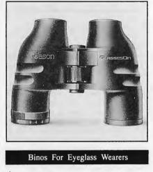
▲ Eyeglass wearers have always had to fumble with their binoculars. Jason Optics has solved this problem by introducing their "GlassesOn" binoculars. Jason extended the eye relief on the instruments so eyeglass wearers may keep on their glasses while using these binoculars.
